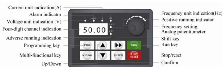
Fig. 4-2 Schematic Diagram of LED Operation Panel
