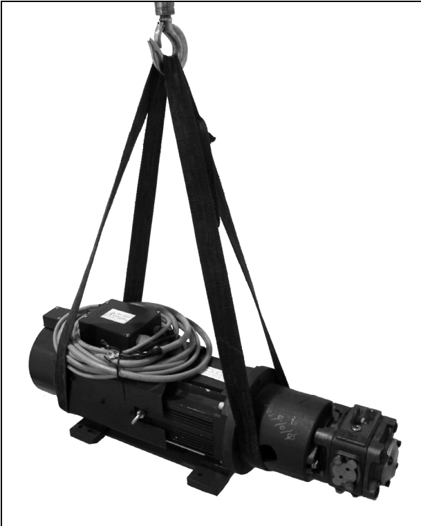
Fig. 11: Lifting the motor-pump assembly (1)
