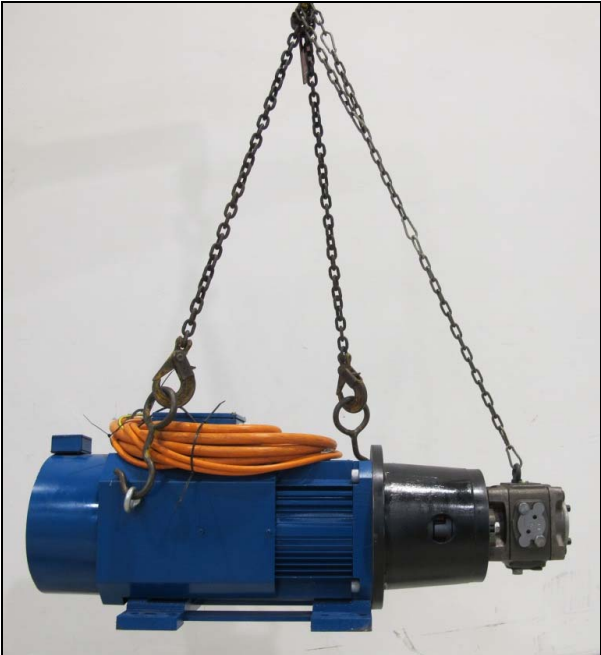
Fig. 12: Lifting the motor-pump assembly (2)
